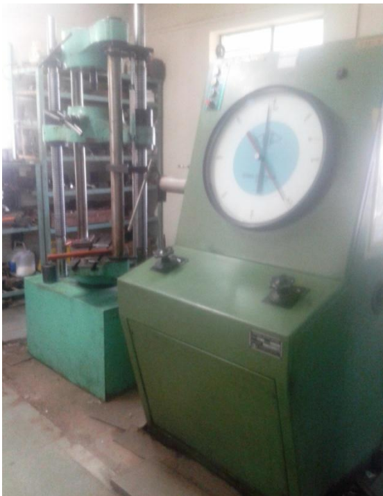
Fig.6 Process Setup for Tensile Test
