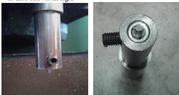
Fig. 3 Friction stir welding taper cylindrical tool with three flutes
