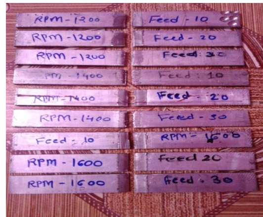
Fig.8 Tensile specimen after failure
