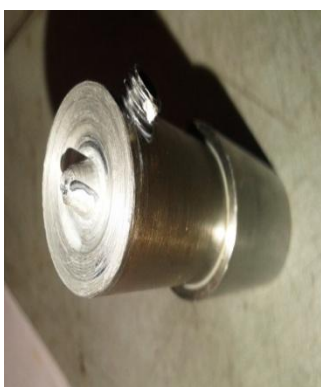
Fig.10 Tool after welding
